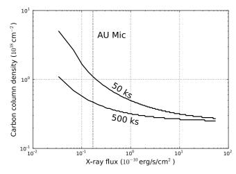
**Fig. B.1.** The detectable carbon column density by measuring the jump height at the carbon edge as a function of the X-ray flux (0.1 keV–2.0 keV). Here, a pure carbon disk is assumed. The two lines represent a 50 ks and a 500 ks exposure with the LETGS. The same temperature structure as AU Mic is assumed which determines the higher order contribution around the carbon edge. The vertical dotted line indicates the X-ray flux of AU Mic.
