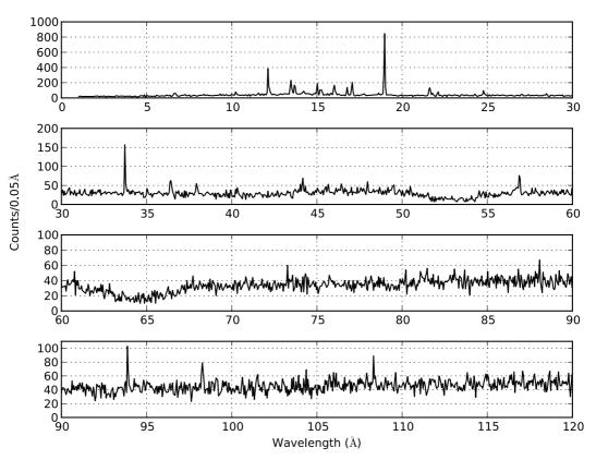
Fig. 3. The measured spectrum in the spectral range relevant for the analysis. Shown is the sum of the positive and the negative diffraction order.
